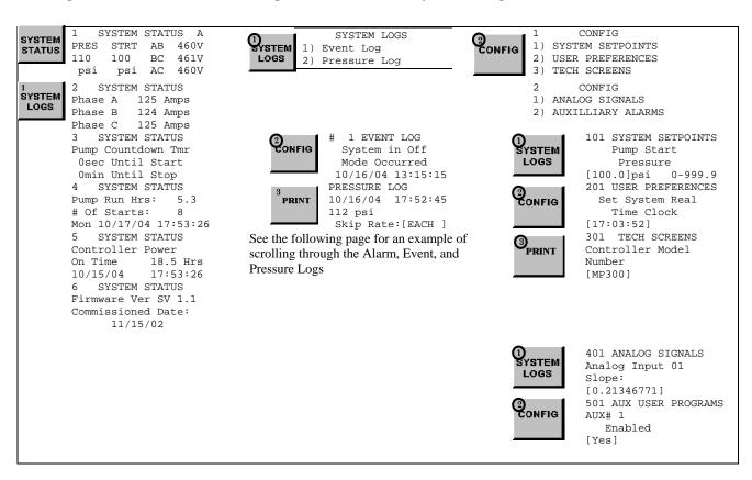
**SYSTEM LOGS:** The Model MP Electric controller has two separate data logs; 1) event log, and 2) pressure log. The event log records all alarm and system function type events. The pressure log records the system pressure at periodic intervals.
